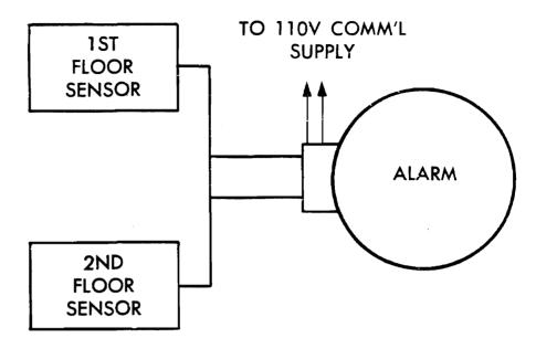
is no power to the alarm system OR the sensing lines fail. There will be no power if the power line fails OR the commercial power is cut off at the source.
